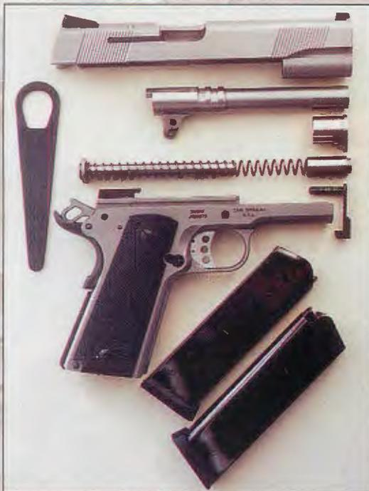
Here, the fieldstripped SW1911 is seen. The pistol comes with two eight-shot magazines and a barrel-bushing wrench.
